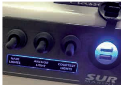
Pannello Surmarine con 2 prese usb Surmarine panel with 2 usb ports
