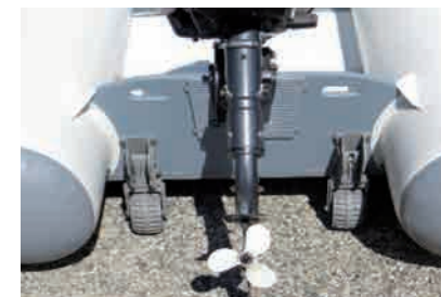
Option: Ruote ribaltabili per gamma "LT" Tilting wheels for gamma "LT"
